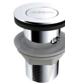
91102-1C-I011 Turnover drainer Ø61*85mm Installation aperture: Ø44mm External thread: G1'1/4
