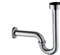
9107-1C-I011 Urinal drain pipe Pipe diameter: Ø32mm OD of flange: Ø65mm Distance between wall & inlet: 240mm Material: copper alloy
