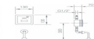
5211-1B1-1 Urinal sensor flushing device 130*130mm Infrared sensing DC power
